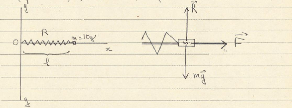
$$F = m\gamma \quad \left. \begin{array}{l} \\ \end{array} \right\} \Rightarrow F = m\omega^2 r$$
