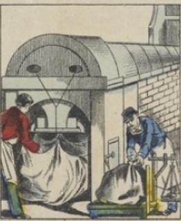
The tobacco leaves are then sent to the TORRÉFACTEURS, large rotating ovens, where they are dried and prepared for smoking. The tobacco is then sent to the APPAREILS DE PAQUETAGE.
