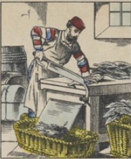
Tobacco arrives in bales or in tonneaux in the factories. The leaves are gathered in groups, more or less large. These packages of leaves are called MANOQUES. The first work consists of cutting the stems to keep the leaves from deteriorating.
