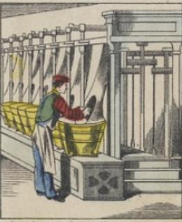
The tobacco is then sent to the MOULINS, where it is ground to a fine powder. However, it is necessary that the powder is not too fine. Therefore, it is sieved. The powder is then sent to the TAMS.
