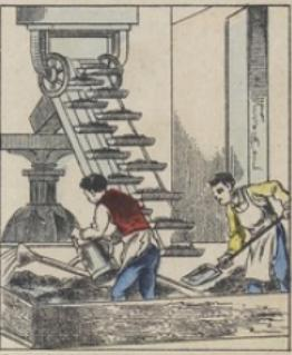
The powder of tobacco is then submitted to a MOULADE of water. This mixture is then sent to the MORIA which磨碎 and then poured into the tanks.
