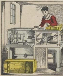
Before being put on sale, each package passes through the MACHINE À PESER, a small and intelligent device invented by the engineer Darquier. Each package weighs TROP or TROP PEU and is rejected by the machine and returned to a new packaging.
