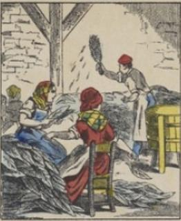
To separate them without breaking them, the leaves of tobacco which are found joined together are pressed in the bales, then sprayed with water with a spray gun. This humidification facilitates the ÉPOULARDAGE or separation and cleaning of the leaves.
