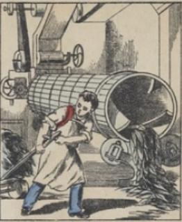
I<sup>e</sup> TABAC À PRISER. The tobacco destined for this fabrication is mixed and moistened with additional water in a MOULIN MÉCANIQUE, an operation whose purpose is to increase their taste and aroma. Then, these leaves are cut into small pieces by HACHOIRS.
